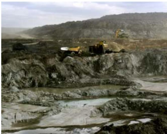
*Open pit mining uses shovels and large trucks to remove oil sand -- a thick and sticky form of crude oil -- in Fort McMurray, Canada. (Photo by Melina Mara/The Washington Post, reproduced with permission.)*
